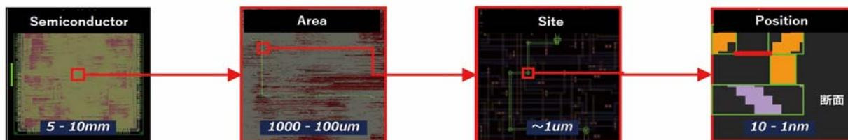
Failure analysis flow
