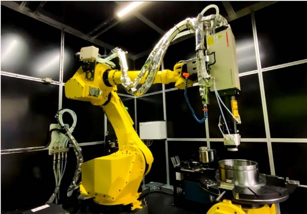
External view of our newly developed laser thermal processing equipment
