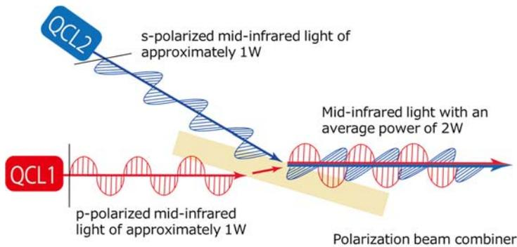
The newly developed polarization beam combiner is used to boost output power by spatially combining mid-infrared light with different polarization angles emitted from two QCLs.
