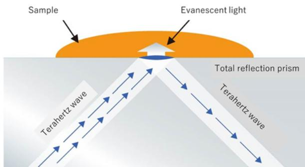
When terahertz waves are totally reflected inside a prism, the small amount of light exuding from the prism is known as evanescent light. The crystallization and moisture content of a sample placed on the prism surface can be measured by detecting the reflected terahertz waves attenuated by the interaction between the evanescent light and the sample.
