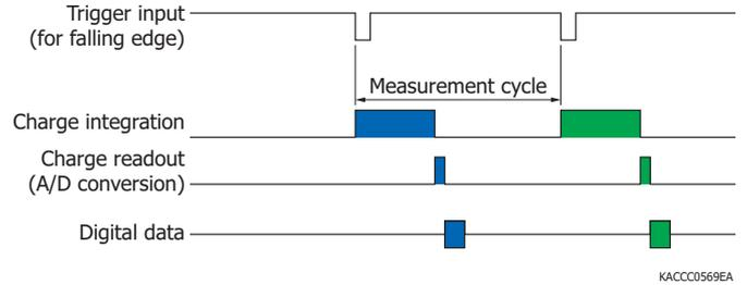
(5) Asynchronous data measurement at external trigger input level
