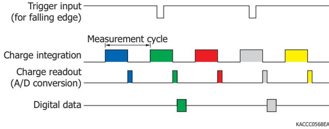
(4) Synchronous data measurement at external trigger input
