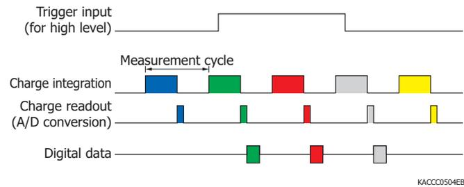
(6) Synchronous data measurement at external trigger input level
