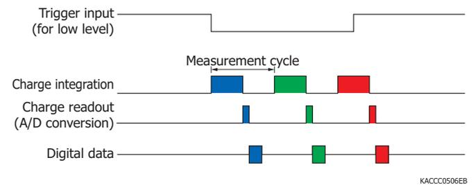
In any of the modes (1) to (6), if the trigger input cycle is shorter than the measurement cycle of the spectrometer, the input trigger is ignored.
