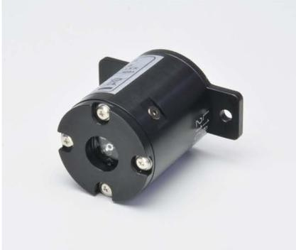
This is a module with built-in lamps and an optical fiber for doing diffuse reflection measurement in near-infrared spectrophotometry. With this product, in which plural lamps and an optical fiber are arranged close to each other, the weak diffused light emitted from the sample can be detected efficiently.
