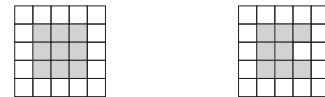
This is defined as defect cluster. This is not defined as defect cluster.
