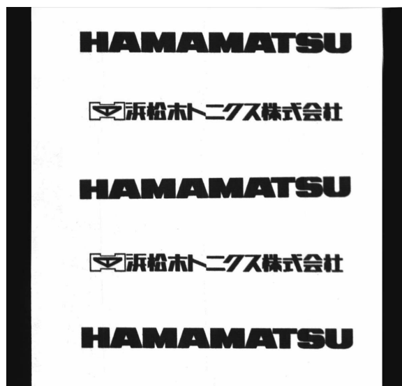
[Figure 1-24] Imaging in TDI operation (continuous image during drum rotation)
