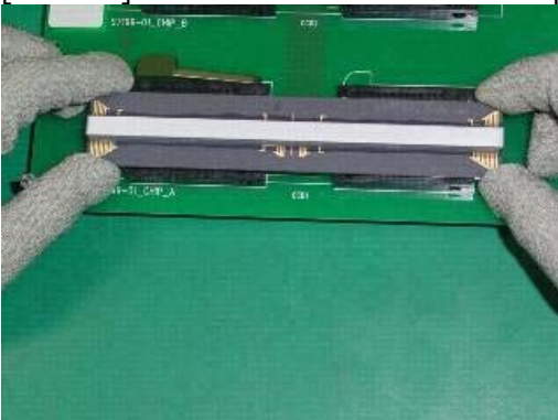
[Photo 7] Press the board to insert the product.
