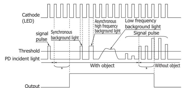
\* A signal is judged to be present only when synchronous detection is carried out three consecutive times, and no signal is judged to be present when synchronous detection is not achieved three consecutive times.
