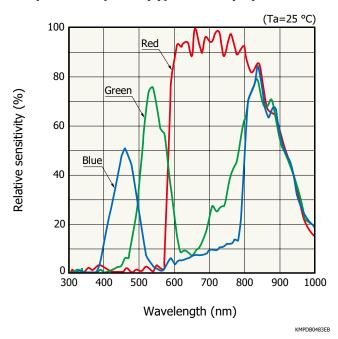
Note: This sensor also has sensitivity in the infrared region, so cut off infrared light as needed.
