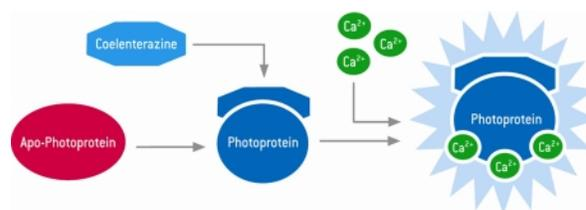
**Fig. 1: Mechanism of the i-Photina reaction**
