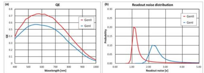
Figure 1: Quantum efficiency (QE) curve and readout noise distribution. For Gen I-sCMOS, the readout noise is shown in global shutter mode.
