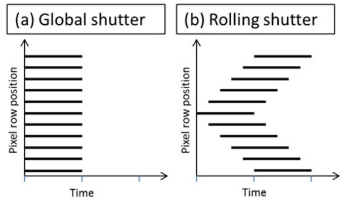
Figure 2: Exposure timing by pixel row position
