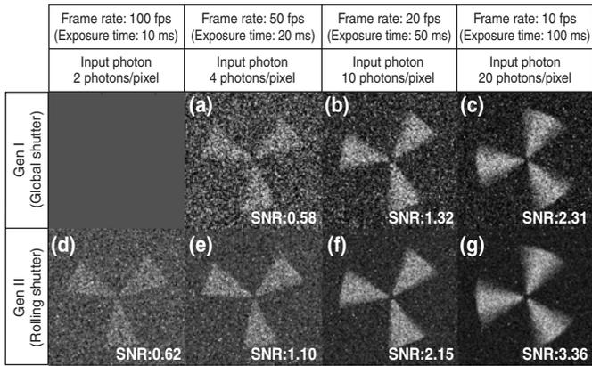
Figure 4: Rotating fan simulation images with camera sensitivity and noise taken into account
