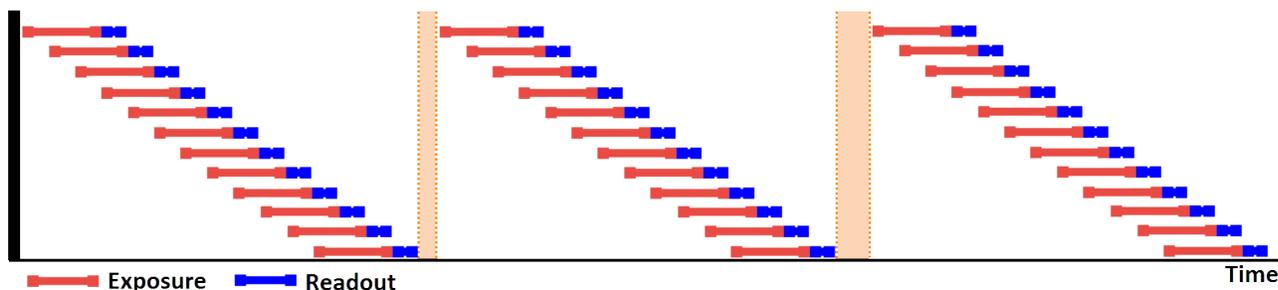
**Internal Line Interval** - Is the readout slope, i.e., the period of time between the readout of two lines. The internal line interval is reported in seconds and can range from 9.7  $\mu$ s to 100 ms.
