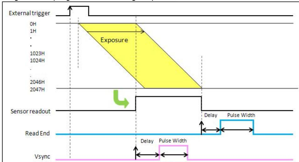
When you choose Hsync for the reference of programmable timing output, the camera can output a number of pulses before the start of exposure. This is called as Pre-Hsync. The Pre-Hsync range is 0 to 2047.
