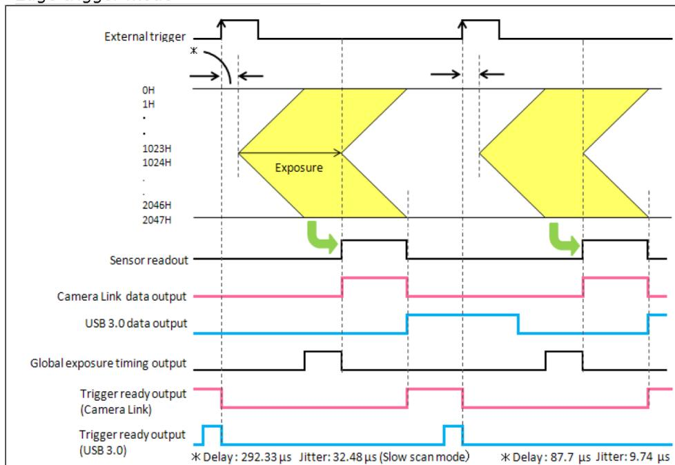
External Edge and Level Trigger: Maximum Speed = Exposure Time + Readout Time
