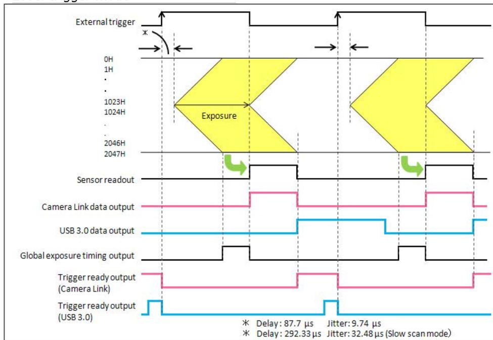
**Note:** In External Level Trigger mode, the exposure time in the Camera Control panel is grayed out because the exposure time is controlled by an external source.
