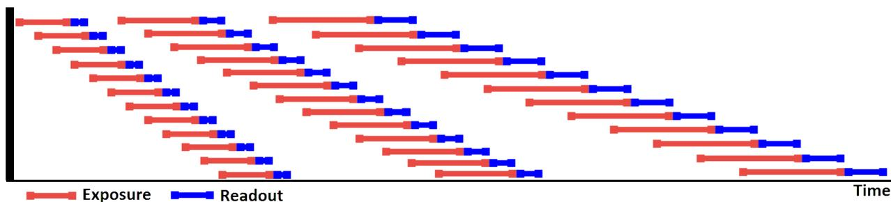
**Internal Line Speed** - Is the vertical speed from top to bottom or bottom to top of the sensor readout. The internal line speed is reported in meters per second and can range from 0.0065 to 0.667 meters per second.
