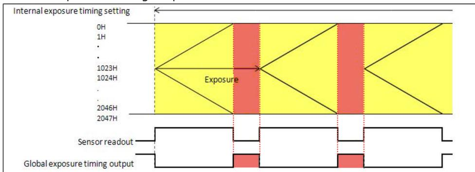
**Note:** There is no output signal when the exposure time is less than the frame rate.
