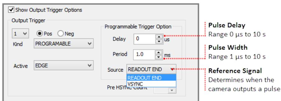
The relation between the parameter which can be set with each reference signal, and an output signal becomes below.
