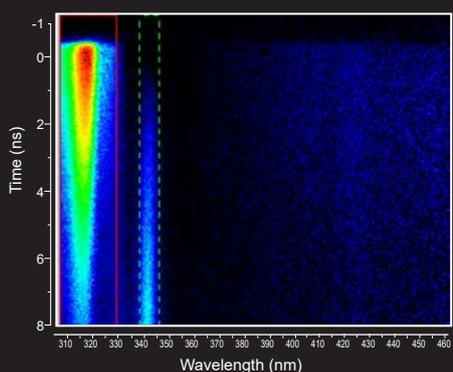
Time-resolved transient absorption spectral streak image in simultaneous observation of the singlet-singlet absorption and the triplet-triplet formation of Anthracene solution
