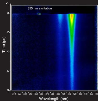
Time-resolved transient absorption spectral streak image of the triplet-triplet absorption of anthracene in supercritical carbon dioxide (40 °C, 10.9 MPa)
