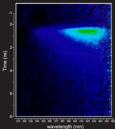
Time-resolved transient absorption spectral streak image of the singlet-singlet absorption of C60
